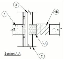
1. **Floor or Wall Assembly** — Min 4-1/2 in. (114 mm) thick reinforced lightweight or normal weight (100-150 pcf or 1600-2400 kg/m³) concrete. Wall may also be constructed of any UL Classified **Concrete Blocks\*.** Max area of opening is 384 in. (2477 cm²) with a max dimension of 32 in. (813 mm).
