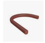
**ZZ**<sup>®</sup> **530 Fire Protection Joint Seal** is simply pushed into the joint from both sides with the prescribed excess dimensions. Through its elastic structure it can compensate elongation movements up to 25%. Alternatively, as closure, in addition a sealant can be applied (e.g. silicone OTTOSEAL S 115 or acrylic OTTOSEAL A 207).
