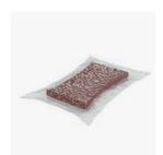
**ZZ**<sup>®</sup> **230-144-V** Fire Protection Block, vacuum-packed can be used for easier sealing of narrow residual openings. After opening the foil, the vacuum-packed Block expands to standard size. The foil can remain in the bulkhead after expansion.
