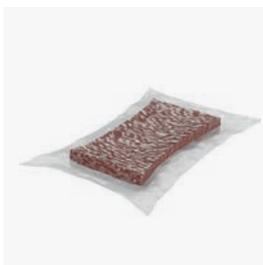
**ZZ® 230-144-V Fire Protection Block**, vacuum-packed can be used for easier sealing of narrow residual openings. After opening the foil, the vacuum-packed Block expands to standard size. The foil can remain in the bulkhead after expansion.
