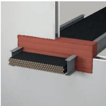
**Cable tray with cables in combination with **ZZ**<sup>®</sup> 360 Fire Protection Foam in drywall (W-L-4085)**
