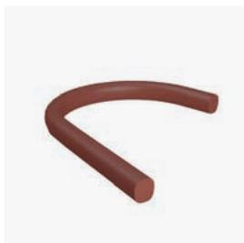
**ZZ® 530 Fire Protection Joint Seal** is simply pushed into the joint from both sides with the prescribed excess dimensions. Through its elastic structure it can compensate elongation movements up to 25%. Alternatively, as closure, in addition a sealant can be applied (e.g. silicone OTTOSEAL S 115 or acrylic OTTOSEAL A 207).
