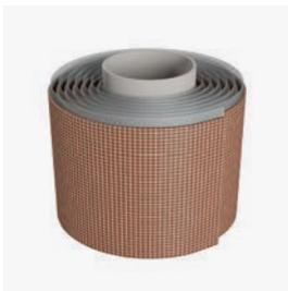
**ZZ® 451-150 Fire Protection Wrap** is a non-shrinking, solvent-free, self-adhesive, plastic butyl sealing tape that is intumescent in the event of fire. It is used as a cable wrap for fire resistance class EI 120 in the system **ZZ® M30**.
